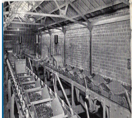
Above the overhead storage hoppers. Showing coal being discharged from the overlapping bucket conveyors by means of the fixed dumpers
